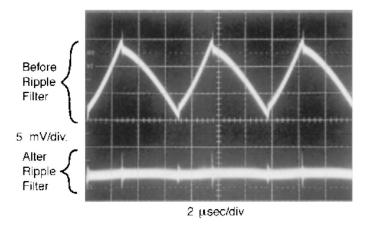
Figure 29. Post Ripple Filter Waveform
