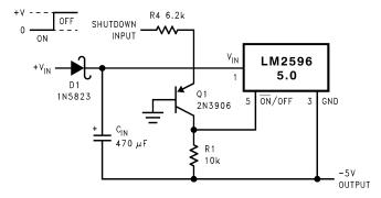
Figure 39. Inverting Regulator Ground Referenced Shutdown
