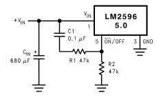
Figure 33. Delayed Startup
