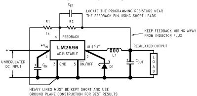
$$\begin{aligned} v_{OUT} &= v_{REF} \left( 1 + \frac{R_2}{R_1} \right) \\ where \ V_{REF} &= 1.23V \\ R_2 &= R_1 \left( \frac{v_{OUT}}{v_{REF}} - 1 \right) \end{aligned}$$
