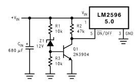
Figure 34. Undervoltage Lockout for Buck Regulator
