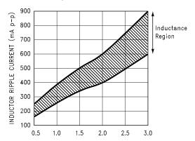
Figure 30. Peak-to-Peak Inductor Ripple Current vs Load Current
