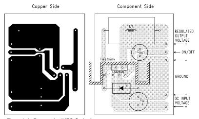
$C_{IN}$ —470 µF, 50V, Aluminum Electrolytic Panasonic, "HFQ Series"  $C_{OUT}$ —330 µF, 35V, Aluminum Electrolytic Panasonic, "HFQ Series" D1—5A, 40V Schottky Rectifier, 1N5825 L1—47 µH, L39, Renco, Through Hole Thermalloy Heat Sink #7020
