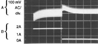
A: Output Voltage, 100 mV/div. (AC) B: 500 mA to 2A Load Pulse
