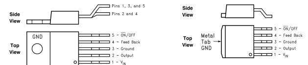
Figure 1. 5-Lead Bent and Staggered Leads, Through Hole TO-220 (T) Package See Package Number NDH0005D
