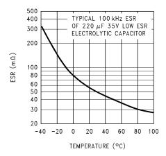
Figure 27. Capacitor ESR Change vs Temperature
