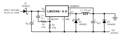
C<sub>IN</sub> —68 μF/25V Tant. Sprague 595D 470 μF/50V Elec. Panasonic HFQ C<sub>OUT</sub> —47 μF/20V Tant. Sprague 595D 220 μF/25V Elec. Panasonic HFQ
