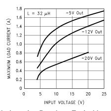
Figure 38. Inverting Regulator Typical Load Current
