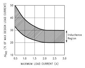
Figure 28. (ΔI<sub>IND</sub>) Peak-to-Peak Inductor Ripple Current (as a Percentage of the Load Current) vs Load Current
